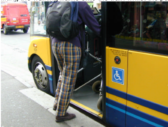
Figure 10: Participant using a walking frame boarding a level-access bus. The proximity to the kerb can be clearly seen.
